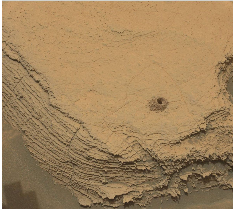
NASA's Curiosity Mars rover used its Mast Camera, or Mastcam, to capture this image of its 36th successful drill hole on Mount Sharp, at a rock called "Canaima." The pulverized sample of this rock was drilled on Oct. 3, 2022, the 3,612th Martian day, or sol, of the mission. NASA/JPL-Caltech/MSSS
