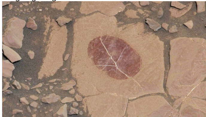
On a part of "Vera Rubin Ridge" where rover-team researchers sought to determine whether dust coatings are hiding rocks' hematite content, the Mast Camera (Mastcam) on NASA's Curiosity Mars rover took this image of a rock surface that had been brushed with the rover's Dust Removal Tool. Credit NASA/JPL-Caltech/MSSS/SSS
